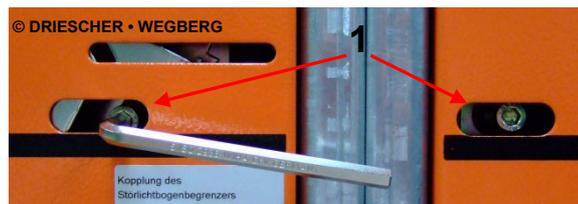
First loosen the two internal hexagonal screws (1) with a hexagonal wrench SW5 to the end stop.
